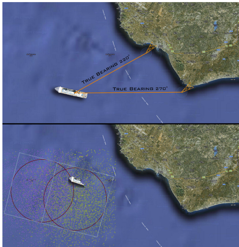
Figure 1: Upper side: a simple scenario with two stations detecting an emergency call. Lower side: datum, search area and probability distribution obtained by the Monte Carlo simulation.
