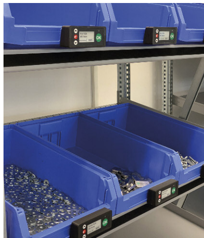
Figure 1: Wireless order handling solutions with the networking technology s-net® by Fraunhofer IIS.
