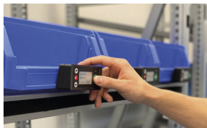
Figure 2: The self-organized radio communication between the individual compartment displays of the pick-by-light system allows an easy installation and is ideally suited for temporary storage structures and rapid remodelling of removal compartments and shelves.
