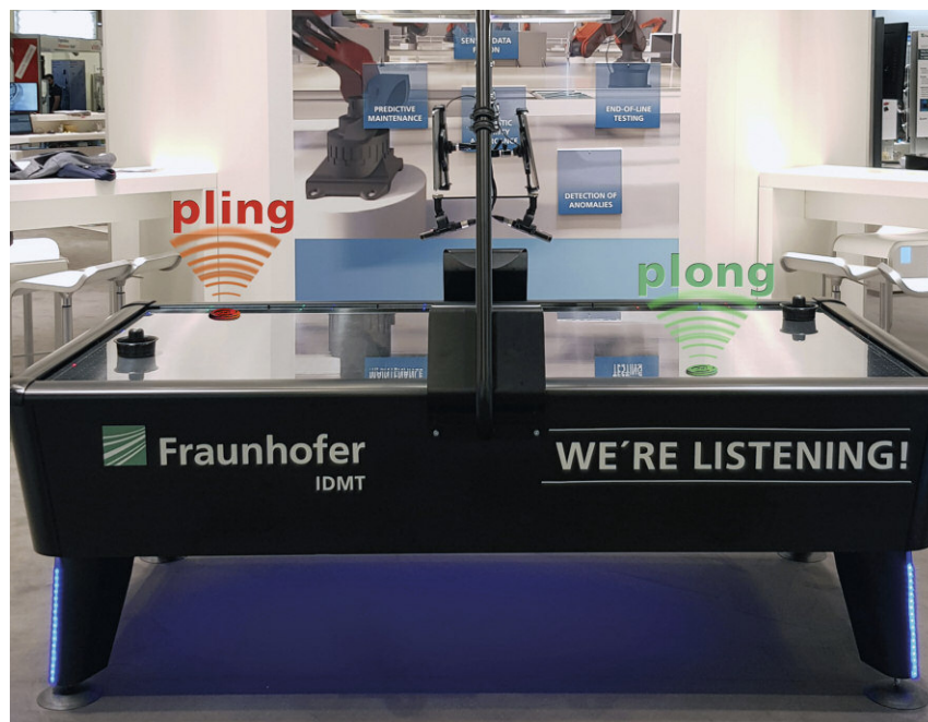
Figure 1: Air hockey table equipped with two measurement microphones recording the puck's sound (e.g., 'pling' and 'plong').
