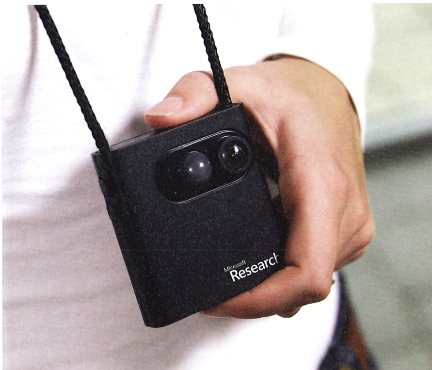
Microsoft SenseCam captures a series of still images triggered by changes in activity (such as movement) and includes sensors that capture other kinds of data (such as ambient light levels and temperature); courtesy Microsoft Research Cambridge.
